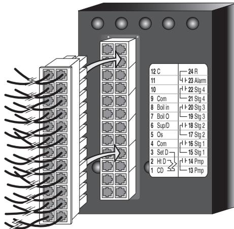
**WARNING:** The BC-1 controller may be pre-wired to the boiler at the factory. Please refer to the appropriate boiler installation and service manual for instructions on electrical connections. If the BC-1 has been pre-wired to the boiler, please do NOT apply power to any of the connections described below (*Powered Input Connections, Output Connections, Sensor and Unpowered Input Connections*).
